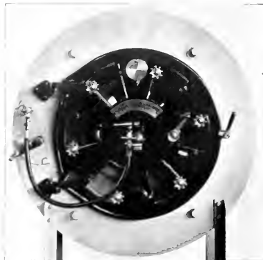
The Morse furnace front arranged for either natural or forced draft.
